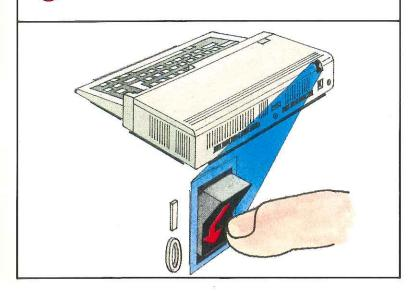
Plug the power cord into the opening marked "P" on the back of the system unit.
